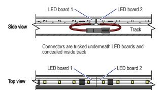
LED boards butt together, ensuring consistent LED spacing and seamless illumination
