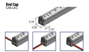
End caps include 3 openings, allowing pigtail leads to feed out of end of fixture as well as to either side of fixture. Allow 3/16" of additional length to fixture for each end cap used.
