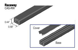
Use to enclose lead wires and splice connections. Low profile and clean shape make raceway inconspicuous and unobtrusive. Made of black PVC. Ships in 5ft sections. Cut to length and miter-cut at corners. Mount base to surface and snap in cover.
